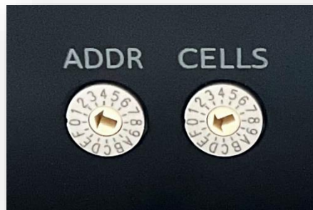
Figure 5: BMS address and cell selection rotary switches.
