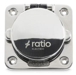
Ratio's Shore Power Inlets MP16, MP32 and M50 are made from solid cast marine grade 316 stainless steel and include an easy locking waterproof cap. The requirements for installation of electrical systems on craft of hull length up to 24m are specified in the ISO13297 standard.
