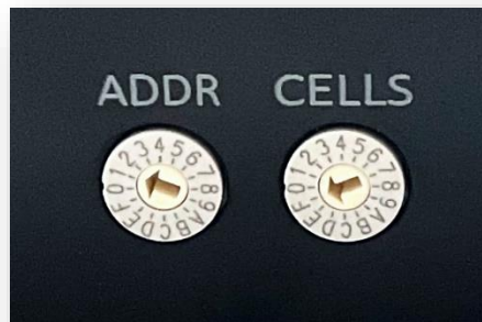
Figure 5: BMS address and cell selection rotary switches.
